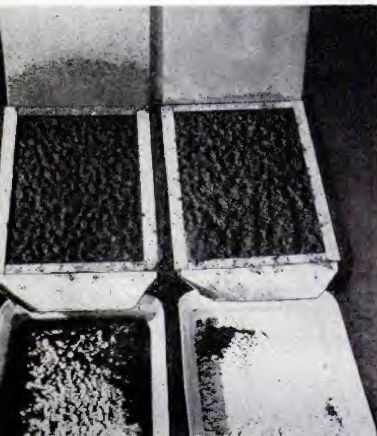
Treated soils were tested under this rain-making machine that duplicates nature's rainfall. Below, soil at left was untreated. Notice the runoff and splatter. Soil in right flat was mixed with Krilium
